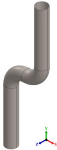
Figure 1: Schematic of a NPS 10 in. SCH 40 STD90° back-to-back pipe bends.
