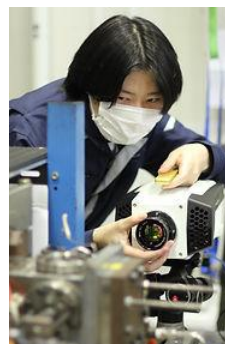
Figure 1: TELOPS FAST M3K enables up to 1.5 – 5.4 \mu\text{m} IR spectral range capture at up to 10 kHz frame rate (left) and wall heat loss mechanism observation settings (right).
