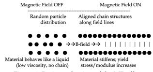
Figure 1: Basic mechanism of the MR effect
