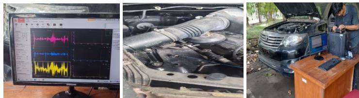
Figure 2: Demonstration on how vibration is captured using sensor and DewesoftX software.
