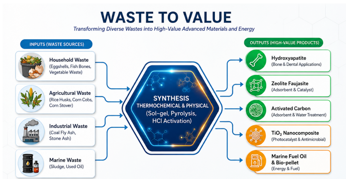
Figure 2: The Waste-to-Value synthesis flow, from waste inputs through thermochemical/ physical synthesis to engineered outputs.
