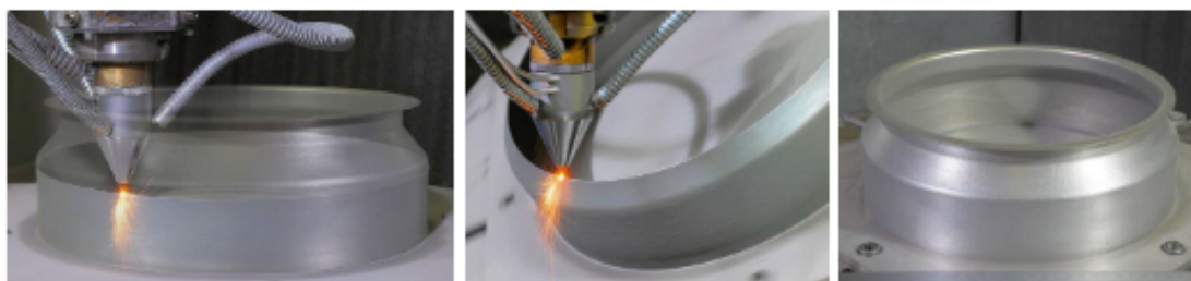
Figure 6: Production of IN718 helicopter engine combustion chamber (courtesy of TWI).
