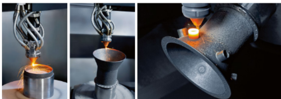
Figure 5: Production of a stainless steel turbine housing (courtesy of DMG Mori).
