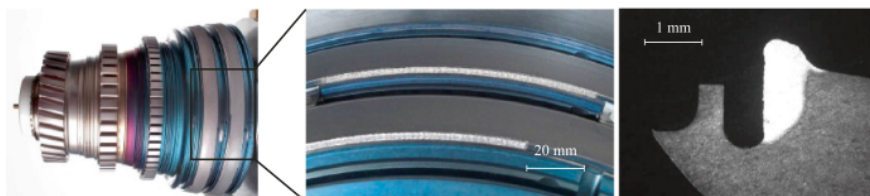
Figure 2: Ti6Al4V groove wall repair using DLMD process (Gasser et al, 2010).
