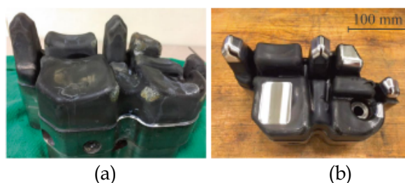
Figure 3: Automotive steel die (a) damaged and (b) restored (Bennett et al, 2019).
