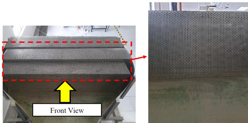
Figure 1: Perforated plate inside water tunnel.
