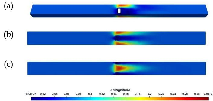
Figure 3: Contour of velocity distribution: (a) domain selection with 2 holes (b) domain selection with 3 holes (c) domain selection with 4 holes.
