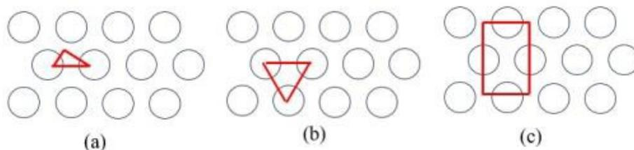
Figure 2: Schematic diagrams for the domain selection from perforated plate (a) domain selection with 2 holes (b) domain selection with 3 holes (c) domain selection with 4 holes.
