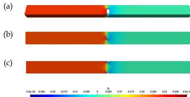
Figure 4: Contour of pressure distribution: (a) domain selection with 2 holes (b) domain selection with 3 holes (c) domain selection with 4 holes.
