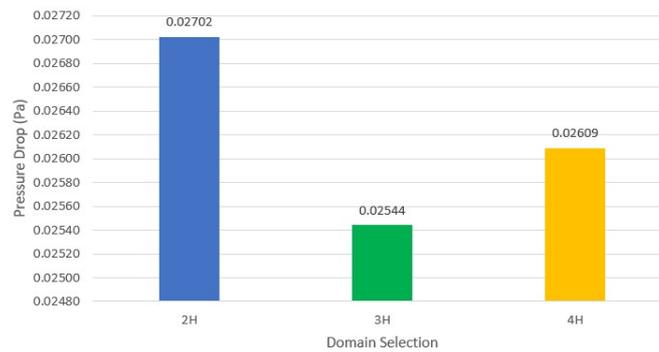
Figure 5: Pressure drop across perforated plate at inlet velocity = 0.0612m/s.
