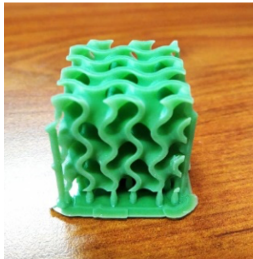
Figure 1: Complete printed Gyroid lattice
