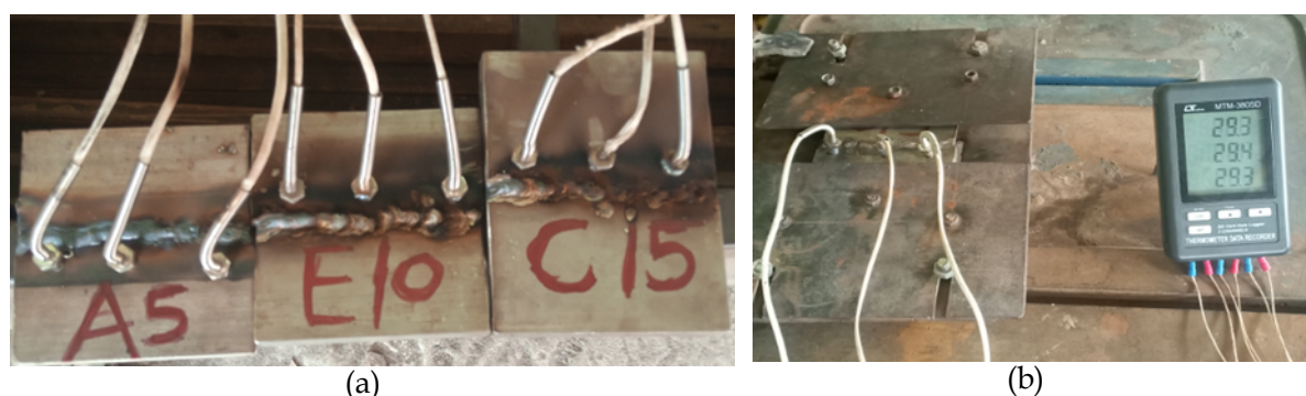
Figure 1: (a) Weld samples and (b) Experimental setup with data logger.
